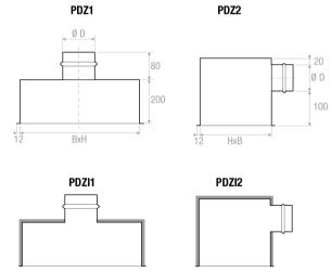
Plenum isolato esternamente spessore 6 mm Plenum externally insulated thickness 6 mm
